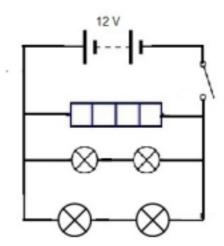
sidelamps remain in series with each other and each pair in parallel with the battery;
